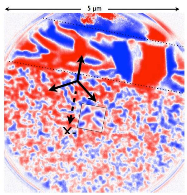
X-PEEM measures surface magnetisation directly. Simulating the image simply involves projecting the simulated magnetisation onto the X-ray direction and convoluting with experimental resolution function (~120 nm in this case).
