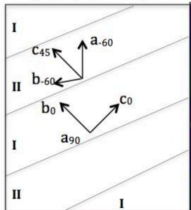
Equilibrium domain structure obtained by micromagnetic simulation.
